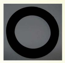
NBR Rubber Gasket Style 9210 is premium grade nitrile, 60 to 85 duro, generally resistance to most hydrocarbon, fats, oils, greases, hydraulic fluids, chemicals and solvents,
