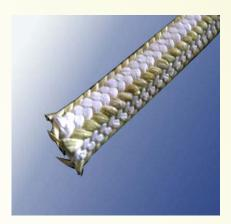
PTFE packing with aramid corners Style 2213 is a braided packing made of PTFE yarns fiber and the reinforced corner yarns of Aramid fiber. This structure enhances the lubrication of Aramid fiber and reinforces the strength of the pure PTFE packing. This special combination packing play a very important role in the sealing of high pressure piston pump.
