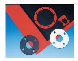
White Silicone Rubber Sheet Style 8950 is special grade silicone, 60 duro, Generally resistant to moderate or oxidizing chemicals, ozone, concentrate sodium hydroxide. ESA, ISO 9001 and FDA Certificates
