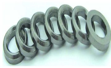
Montero high pressure seal ring made of pure mineral graphite ring from pure exfoliated tape with phosphorus corrosion inhibitor and covered with SS316L top and bottom.
