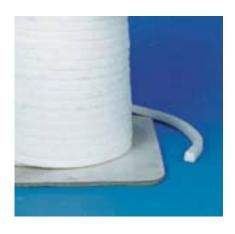
Pure PTFE fiber braided packing with oil style 1132 made of PTFE silk yarns The packing is then re-impregnated with a mix of PTFE and inert lubricant during plaiting operation is a braided packing. It is recommended for chemical engineering, foodstuff, pharmaceutic where contamination is not allowed. Also it can be applied to seal all chemicals except molten alkali metals.
